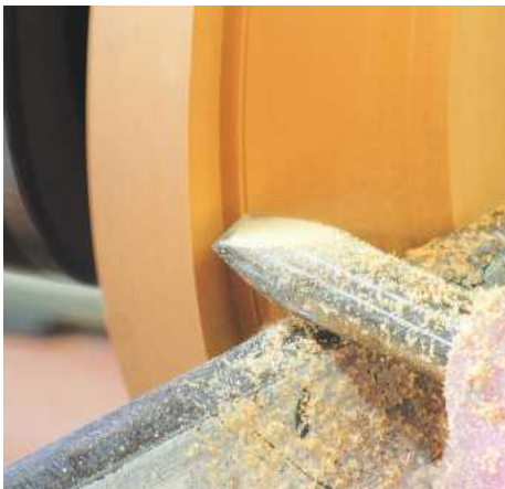
▲ Pic.10 Any detailing such as this small fillet is cut with a skew used in scraping mode. The tool is flat on the rest and gently pushed into the wood
